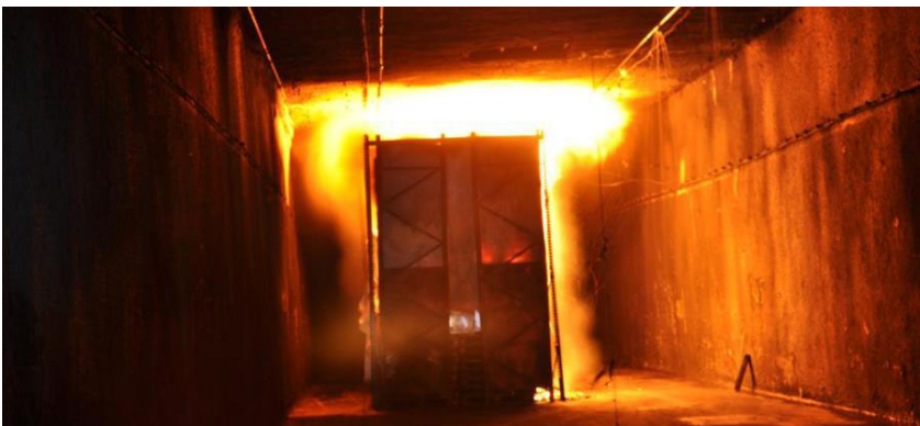
Full-scale fire-suppression test, simulating a fully loaded lorry.
