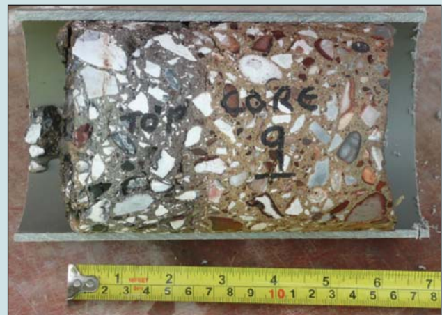
Core 9: taken from the floor to tank 12 bund under an area suspected of receiving a jet of burning fuel. 70 mm thick light grey zone exhibits extreme heating.
