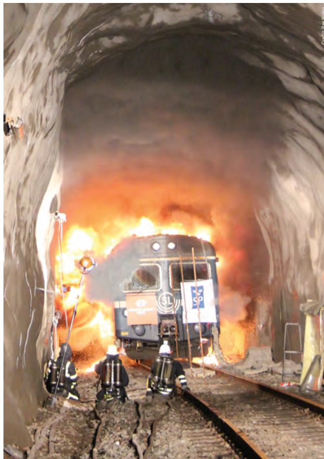
Fire test shot of the METRO project undertaken by Mälardalen University in Sweden
