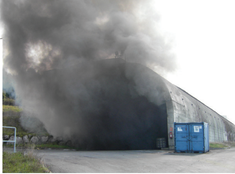
Photo showing full scale fire test carried out by Mosen used to verify its 3D computational fluid dynamics modelling in developing the MoJet vent system
