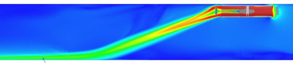
Discharged flow adheres to floor due to Coanda effect
