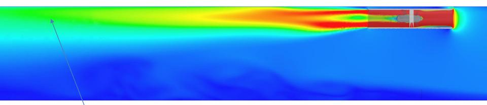
Discharged flow adheres to soffit due to Coanda effect
