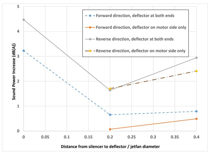
Measurements according to ISO 13347-4:2004 "Industrial fans - Determination of fan sound power levels under standardized laboratory conditions - Part 4: Sound intensity method".
