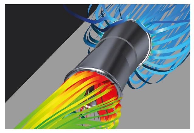
Flow discharged from jet fans exhibits a high degree of swirl, which assists in dissipating the jet and imparting its axial momentum
