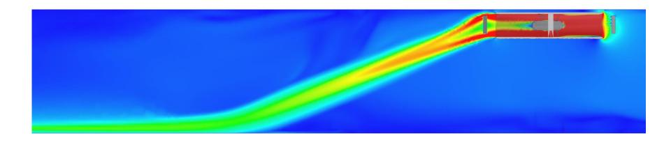
If the jet attaches to the tunnel floor, a dramatic reduction in in-tunnel thrust can occur (installation factor down from 0.84 for a conventional jet fan to 0.60 for a jet fan with deflectors)
