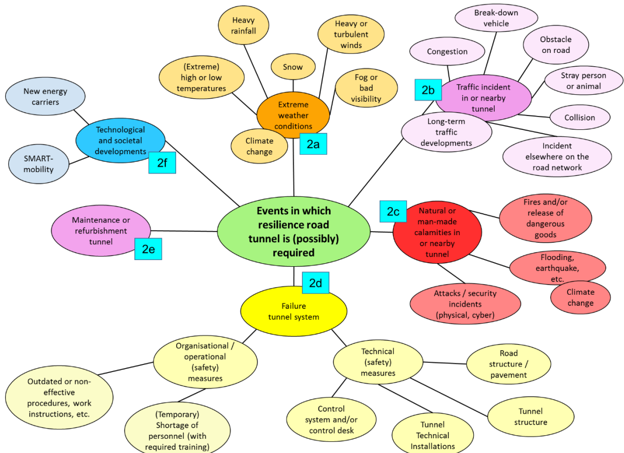
Figure 2. Overview of events or situations in which road tunnel resilience is (possibly) required
