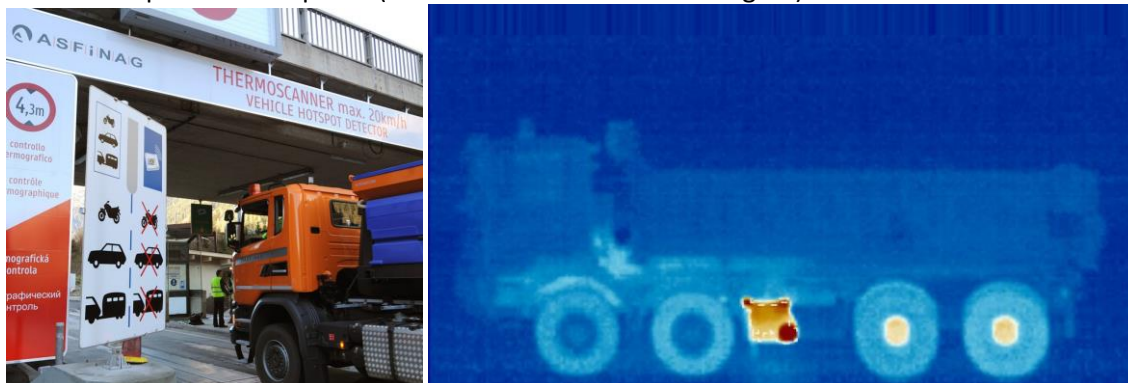
Figure 4: Truck passing a thermo scanner (similar to the one installed at the Karavanke Road Tunnel) and the resulting visualization of the temperature distribution
